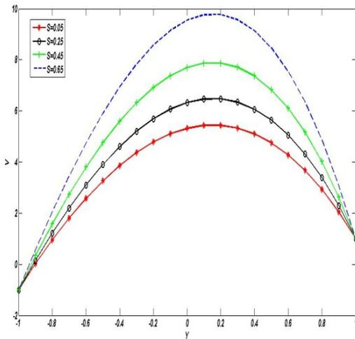
Fig. 2: Velocity profile for different values of  $S$
