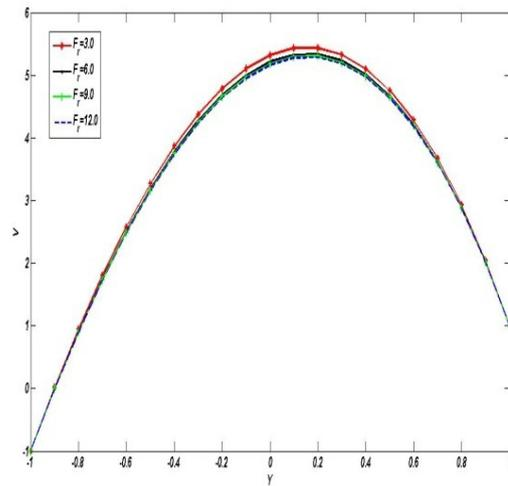
Fig. 4: Velocity profile for different values of  $F_r$
