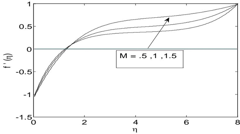
**Figure-3:** Velocity profile for various values of  $M$  when  $\varepsilon = -1.1, Ec=1, m=2/3, S_p = .06$ .
