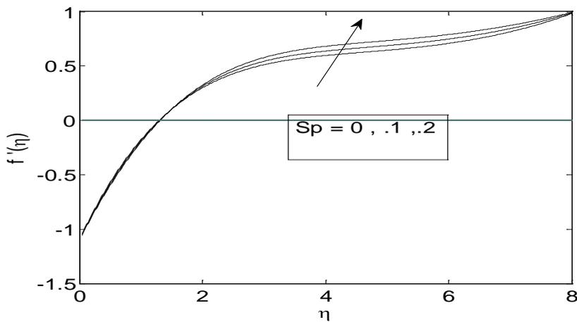
**Figure-5:** Velocity profile for various values of  $S_p$  when  $\varepsilon = -1.1, m=2/3, M=.5$ .
