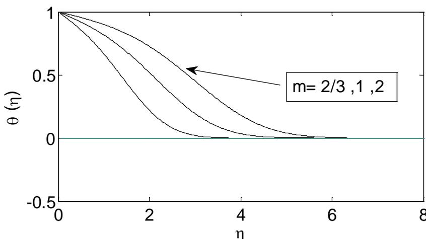
**Figure-2:** Temperature profile for various values of  $m$  when  $\varepsilon = -1.1$ ,  $Ec=0.1$ ,  $Pr=7$ ,  $M=0.1$ ,  $S_p = 0.0001$ .
