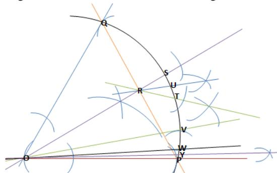
Figure-5: Construction of a  $1^\circ$  angle.
