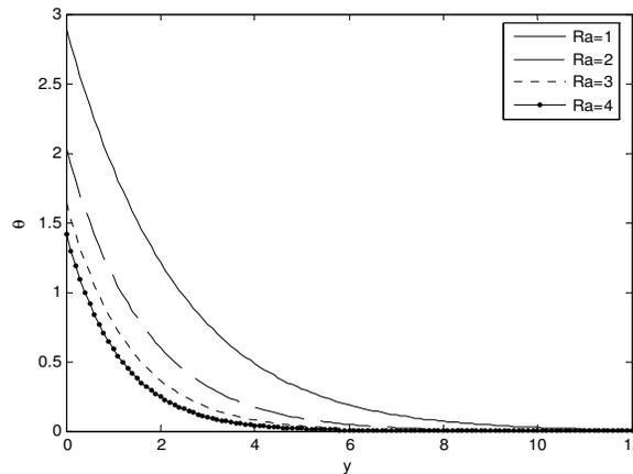
**Fig3:** Temperature distribution  $M=1, Ec=0.01, Gr=5, t=n=1$  with  $\kappa=1$
