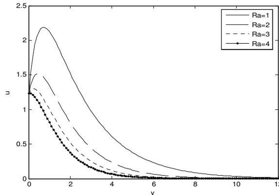
**Fig2:** Velocity distribution, M=1, Ec=0.01, Gr=5, t=n=1 with κ=3
