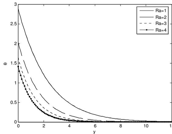
**Fig4:** Temperature distribution  $M=1, Ec=0.01, Gr=5, t=n=1$  with  $\kappa=3$ .
