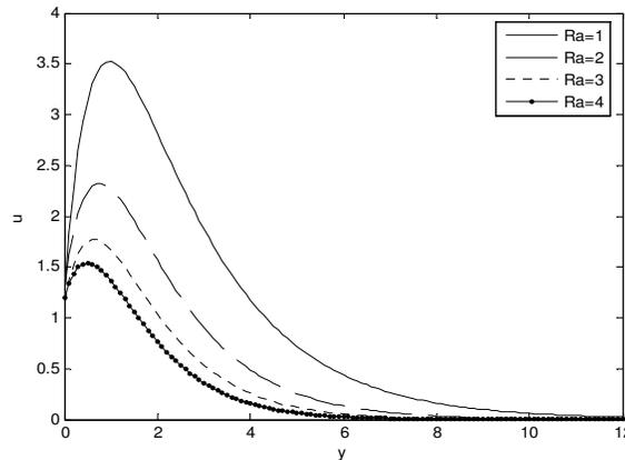
**Fig1:** Velocity distribution, M=1, Ec=0.01, Gr=5, t=n=1 with κ=1
