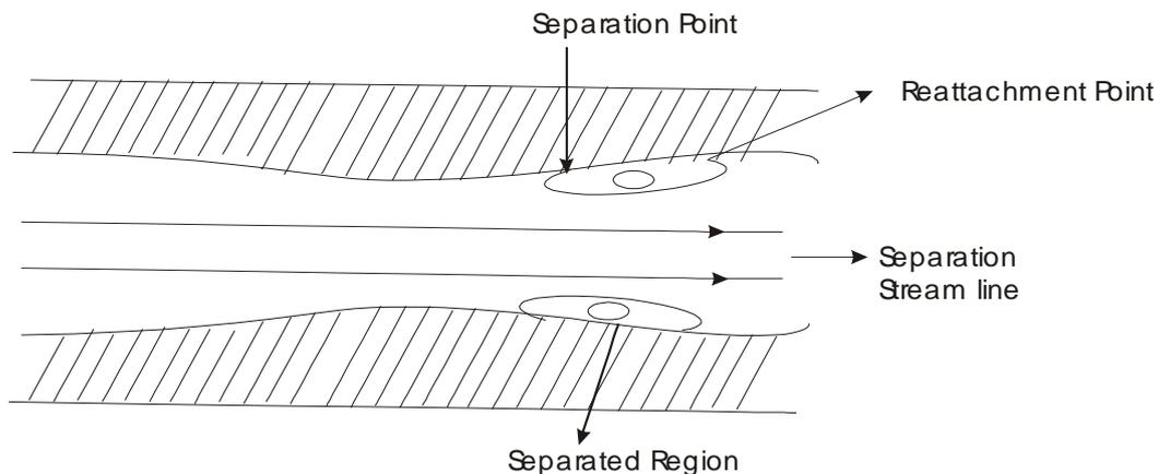
Figure-2: Separation in an axisymmetric stenosis
