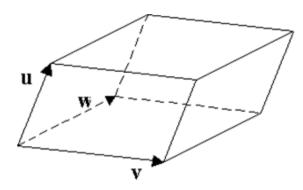
If  $u=(a_{11},a_{12},a_{13})$ ;  $v=(a_{21},a_{22},a_{23})$  and  $w=(a_{31},a_{32},a_{33})$ , then the volume of the slanted box determined by u, v, and w (see picture) is the absolute value of the determinant of the matrix
